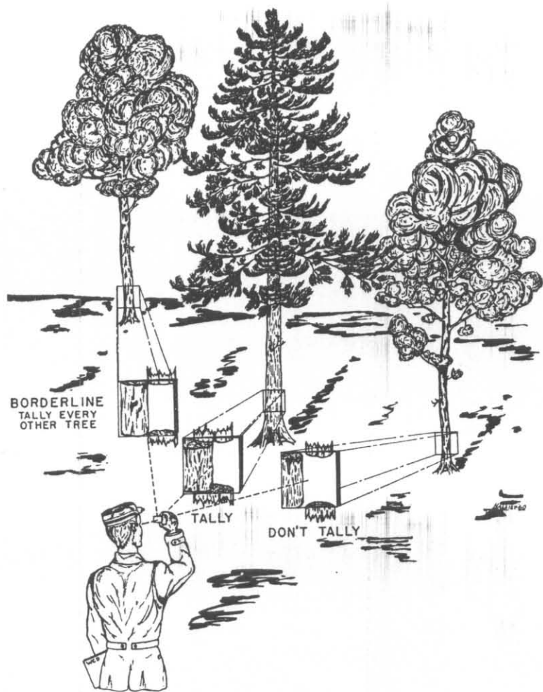
Figure 2. Point-sampling with wedge prism.
